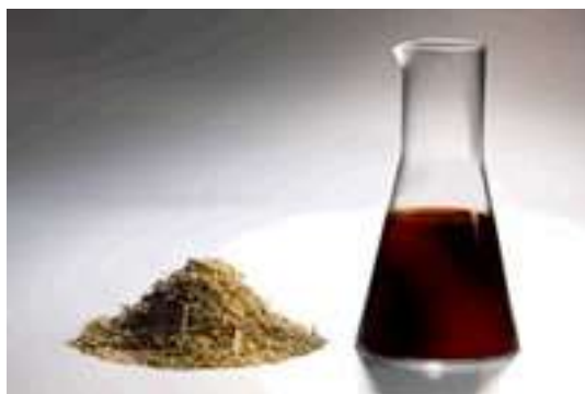
Figure 6. Biomass-based fuel oil by pyrolysis (Source: Metso).
