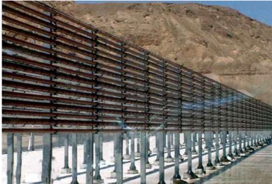
Figure 2-8 H. pluvialis Production in Tubular Photobioreactors (Algatech Corp., Israel)
