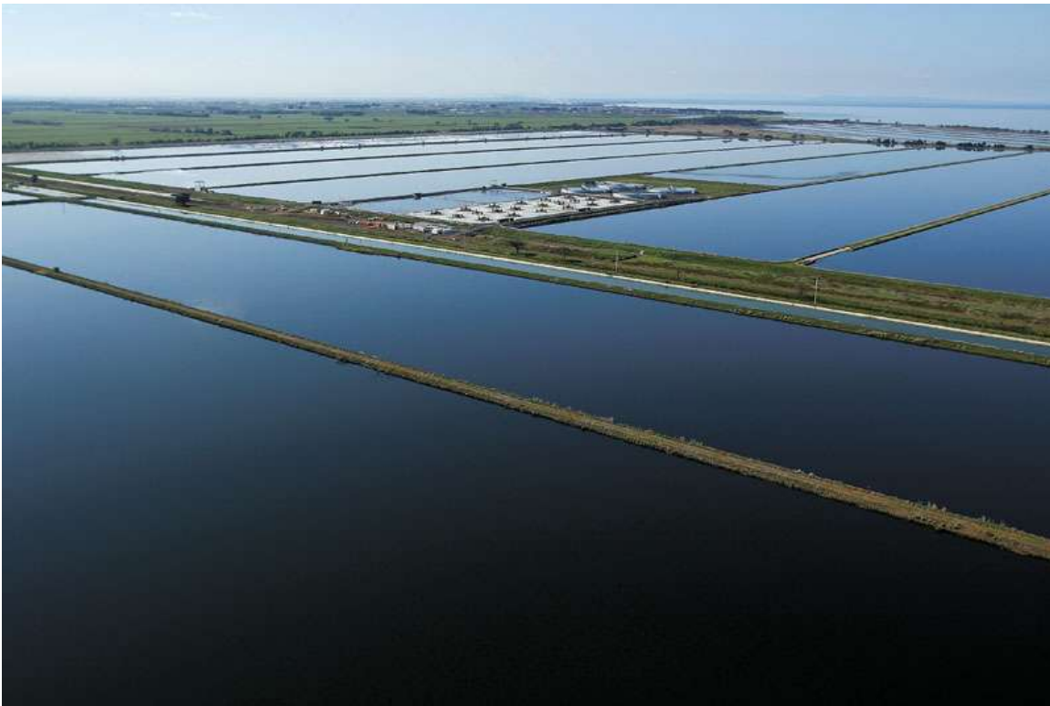
Figure 2-2 Extensive Oxidation Ponds for Sewage Treatment Melbourne Water Corporation's Western Treatment Plant, Werribee, Australia
