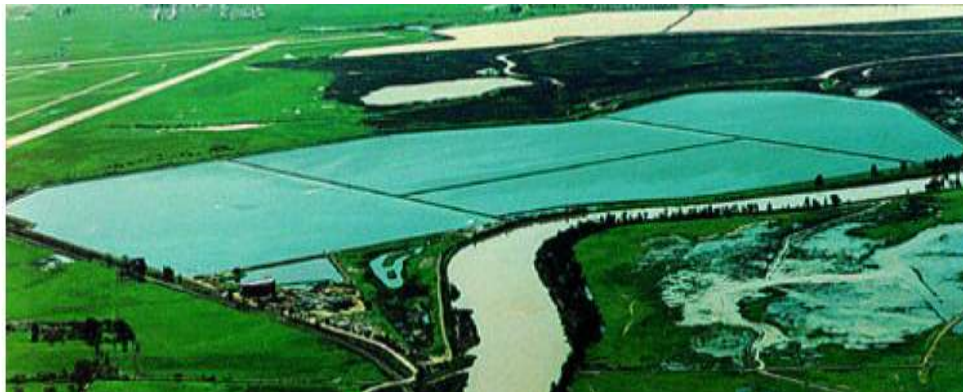
Figure E-2 Typical Oxidation Pond
