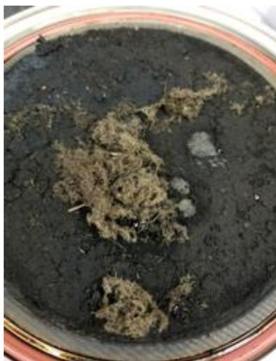
**Figure 30. Filter cake on the 5-micron screen of the ATM-HTL biocrude.**
